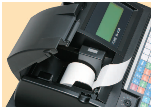
'Drop-in' paper loading mechanism helps users to change paper instantly.
